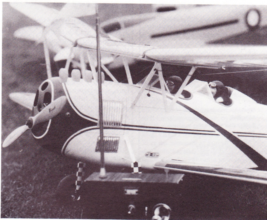
Detail-billede af Great Lakes Trainer. Radioen var en Microprop proportional (single stick), motoren en Merco .49
