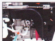
Shrouded-fan for efficient thermal dissipation
