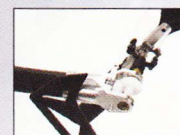
Torque tube driven system for crisp rudder response
