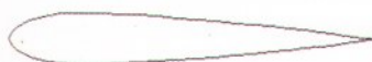
E474 (14.09%) Max thickness 14.08% at 21.5% of the chord Max camber 0.00% at 0.0% of the chord
